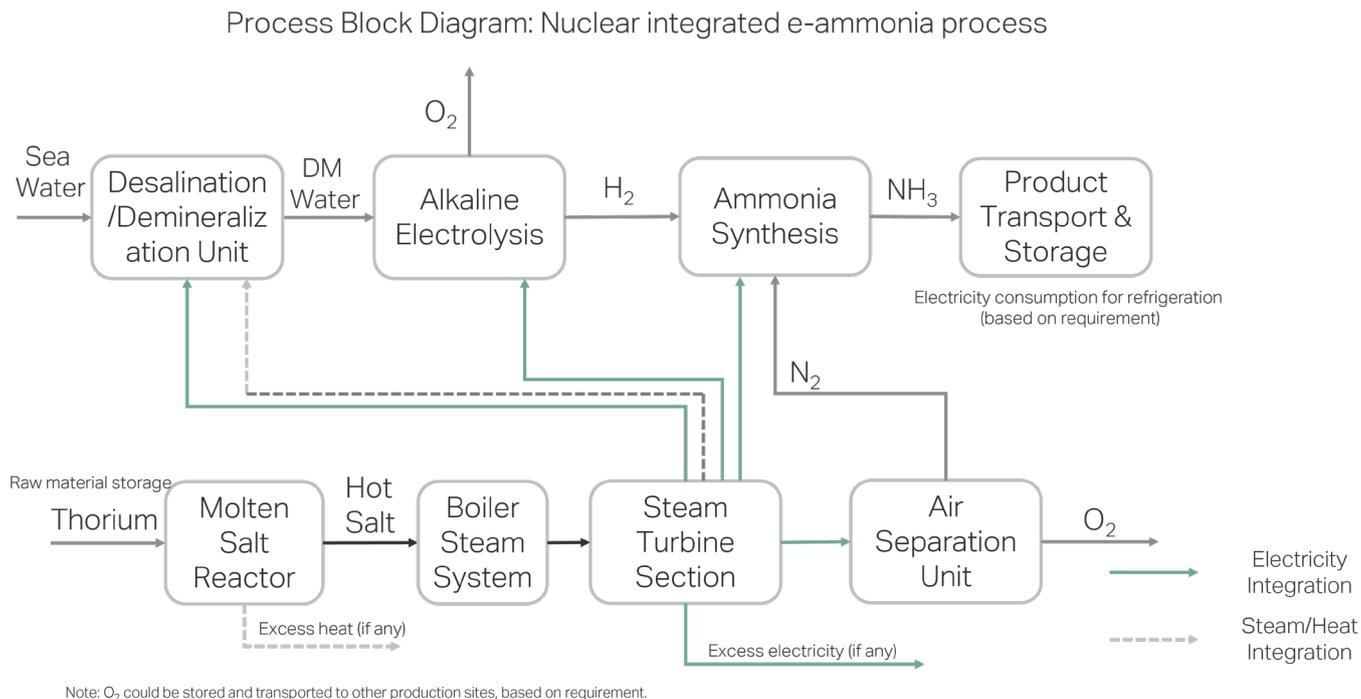
**Figure 2** Block diagram representation of Nuclear based Ammonia production process
