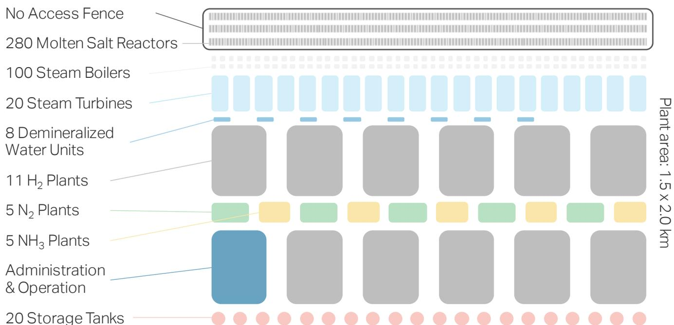
**Figure 3** An indicative depiction of one potential plant layout, to indicate the size of plant components and the land use requirement.
