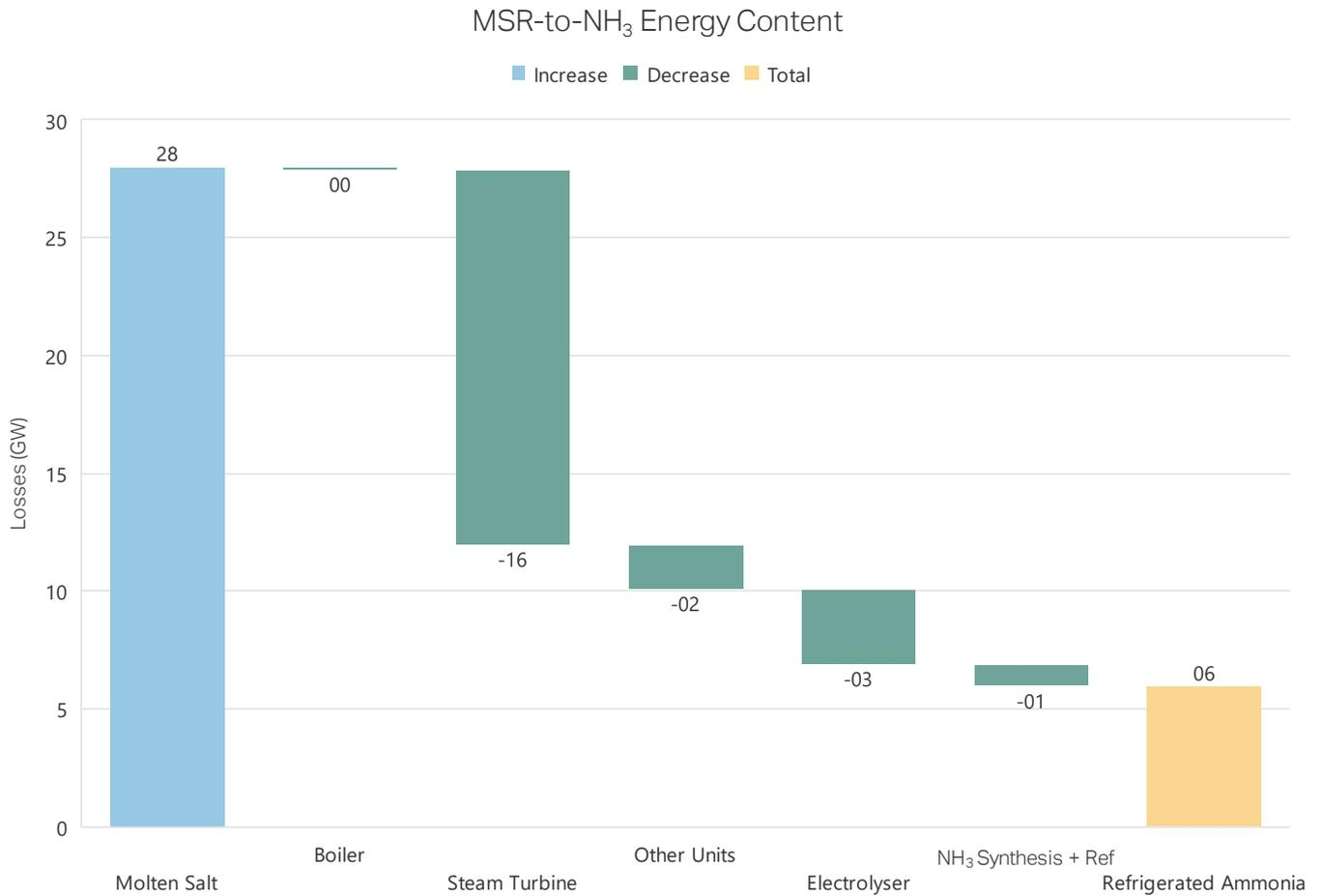
**Figure 4** Overview of energy losses at various conversion steps, starting from molten salt heat power and finishing with ammonia as a fuel pre-combustion.
